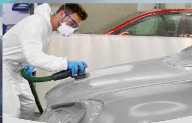
The new air-drying record allows sanding after just 20 minutes depending on local climatic conditions.
